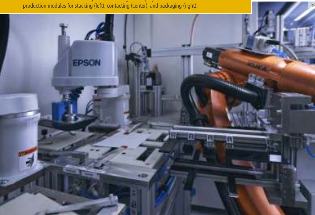
Interior view of the SmartBatteryMaker of the AgiloBat2 project with the central robot and three production modules for stacking (left), contacting (center), and packaging (right).
